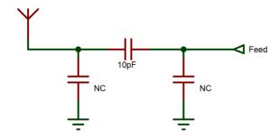
Use of High-Frequency/High-Q Capacitors and inductors is recommended for matching network.
