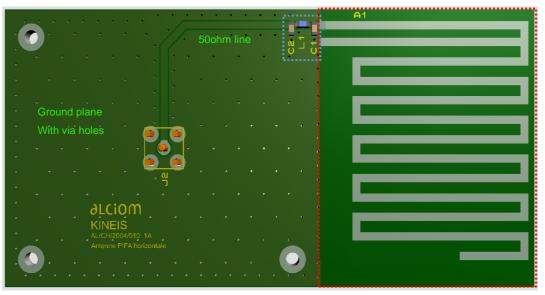
Ground Clearance Area (40 x 50 mm) all metallization should be removed from all layers
