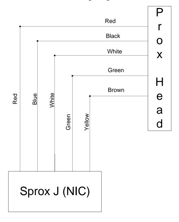
This is a diagram for connecting the SPROX J to the Proximity Head as of 04/10/2013. Please refer to www.interbar.com to verify wiring diagram.
