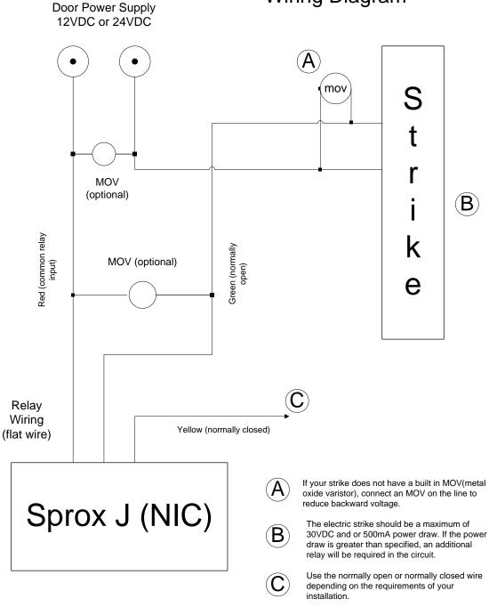
This is a diagram for the SPROX J as of 04/10/2013. Please refer to www.interbar.com to verify wiring diagram.
