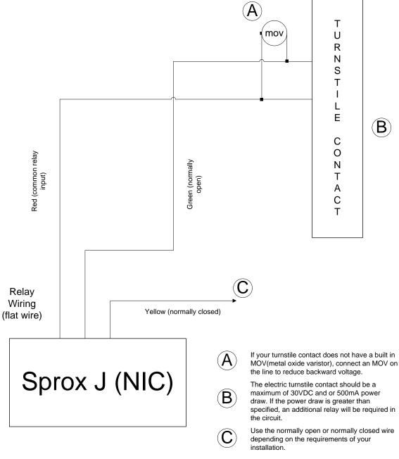
This is a diagram for the SPROX J as of 04/10/2013. Please refer to www.interbar.com to verify wiring diagram.
