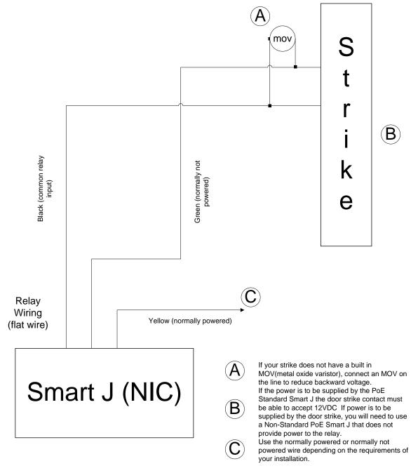
This is a diagram for the Smart J as of 04/10/2013. Please refer to www.interbar.com to verify wiring diagram.
