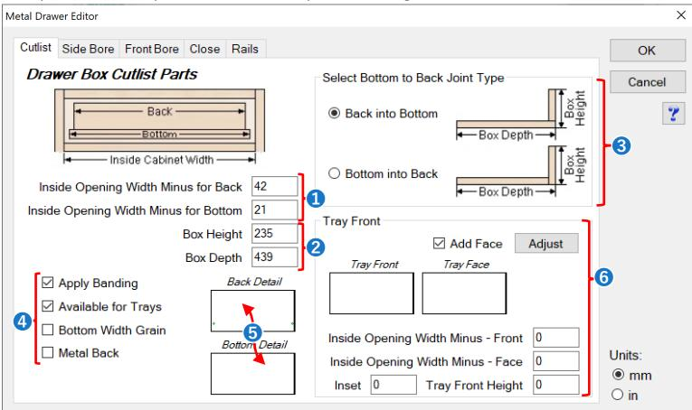
Use the Metal Drawer Editor to set up the dimensions, operations, and options for each height/depth of your metal drawers.
