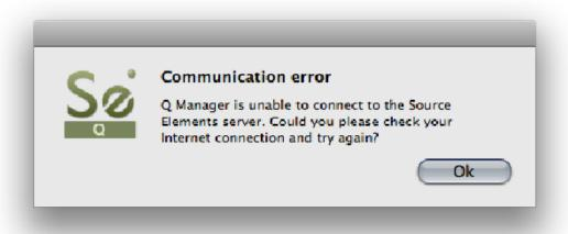
If the Q Manager cannot connect to the internet, perhaps due to a firewall settings or other network configuration issues, the status will be Offline. Check that your internet connection is working, and if you have a built-in firewall you will need to allow access to the Q Manager and Q Daemon.
