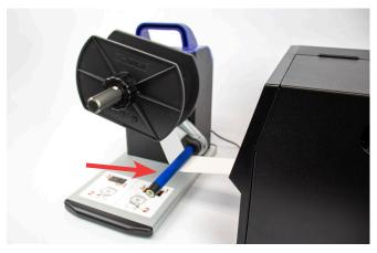
8. Gently push the blue label press bar toward the printer to start label rewinder. Label rewinder automatically stops when labels are wound tight. Move printer for labels to lay flat, if needed.
