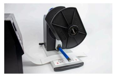
2. Plug power adapter into rewinder and working outlet. **Do not** turn on. Press the feed button of printer to extend labels 10-14 inches.
