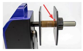
6. Slide the front label stop plate on label rewinding shaft leaving 1 mm space between the cardboard core/edge of labels and the front label stop plate. Slide and push the lock ring knob on the label rewinding shaft and turn clockwise to lock front label stop plate in place.
