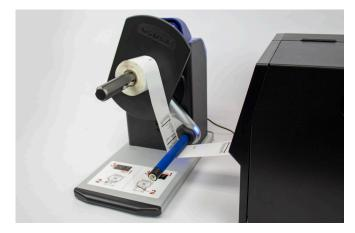
9. Toggle power switch to "O", turning off power, and cut labels near printer. Turn the lock ring knob counterclockwise and remove. Slide the front label stop plate to remove.
