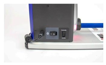
7. Toggle the rewinding switch to "Outside" (wind labels facing outward) and the power switch to "-" to power on, cycle through colored lights to display pink.
