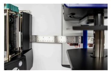
1. Place label rewinder parallel to printer with 5 inch minimum distance. Confirm printer to rewind and label rewinding shaft are in a straight line.
