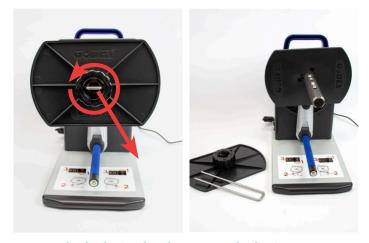
3. Turn the lock ring knob counterclockwise to remove and slide off front label stop plate. Pull paper clip from end of label rewinding shaft to remove. Set both aside.
