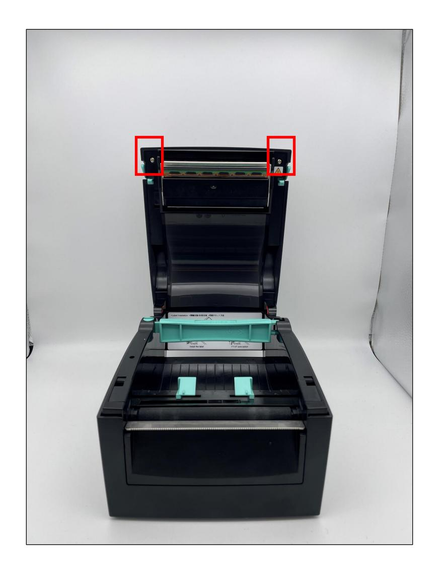
2. Gently close the printer lid but do not latch. Unscrew each screw of the broken release button that needs to be replaced.
