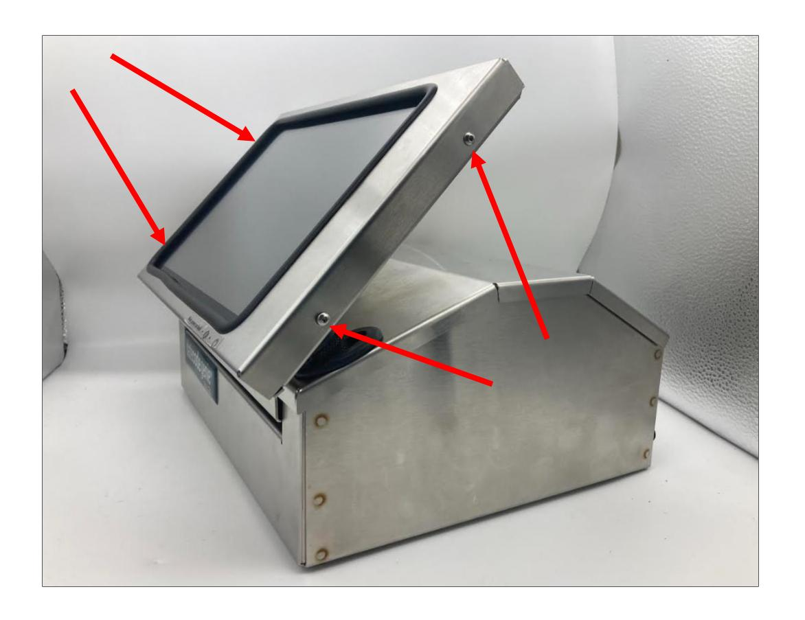
3. Separate the front and back of the tablet frame to expose the tablet.
