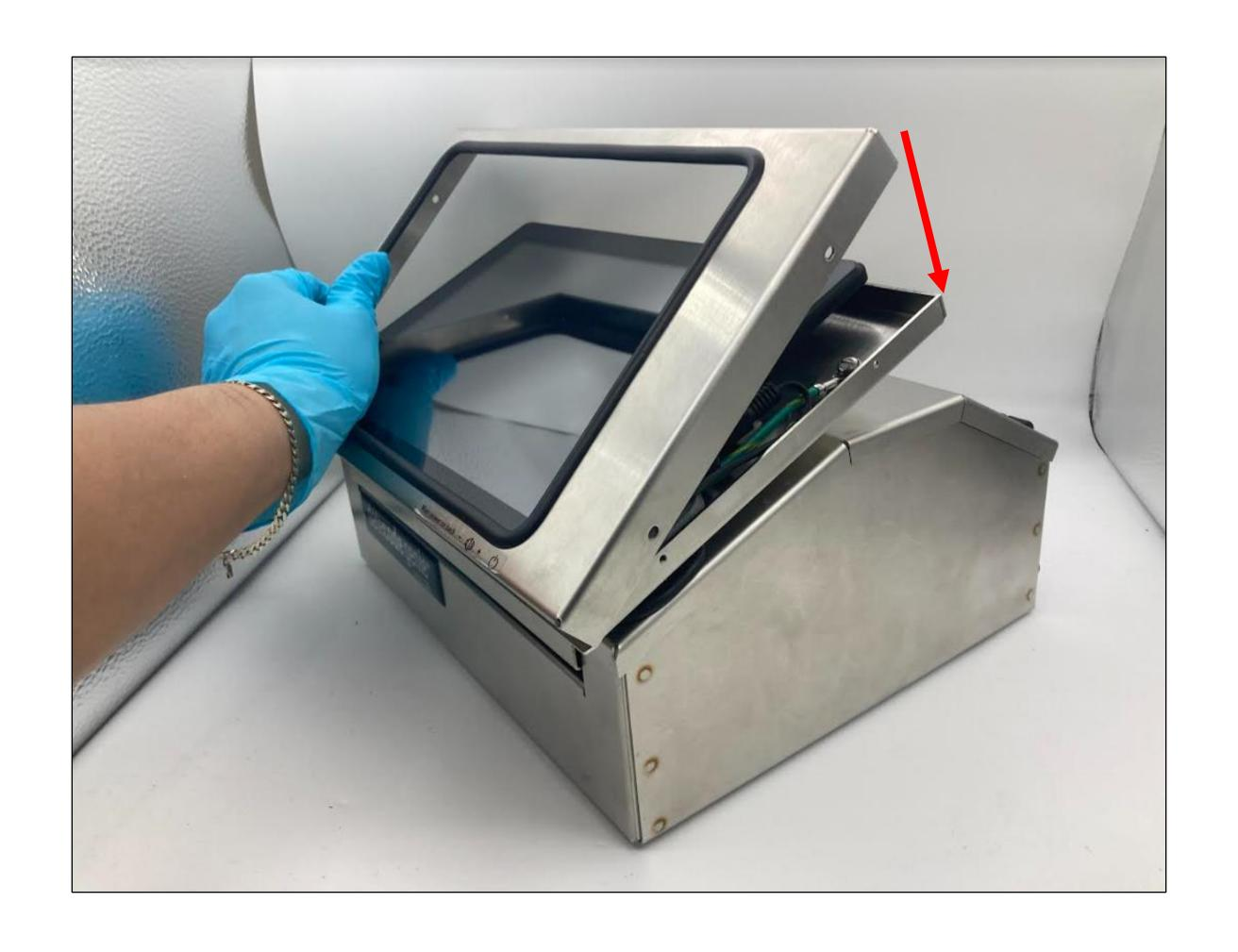
6. Inspect the cables to ensure they are not damaged. Connect cabling to the new tablet as shown.
