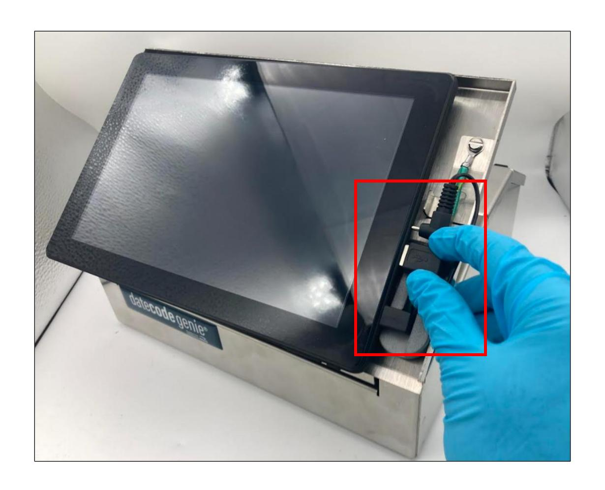
5. Place and reinstall the front tablet frame bottom first.
