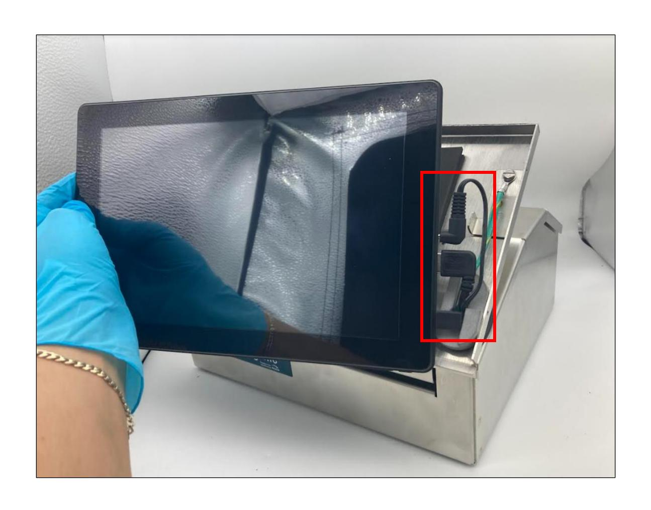
7. Reinsert the four screws on the sides of the tablet frame using the 2 mm Allen head L wrench to tighten.
