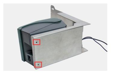
4. Place printer on tray of shelf and lay on side. Line up two holes with printer, insert two screws and tighten with Phillips screwdriver.
