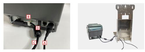
2. Connect the printer by plugging in the power cord A and USB cable C, using the white clip B to secure the cable. Attach the Ferrite clamp D about 1 inch away from the clip to close.
