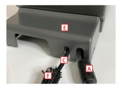
3. Snap the printer cable cover E in place to protect connections. Attach the mesh cable protector F to the USB cable C.
