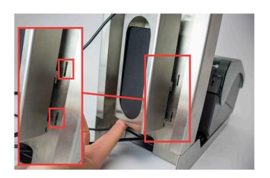
5. Place printer power supply into power supply cover with hooks pointing towards unplugged end. Insert power supply cover hooks into slots on back and gently push down to secure. Plug the other end of the power cord and USB cord into the back of the tablet.
