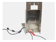
1. Feed the printer power cord and USB cable through the bottom opening.
