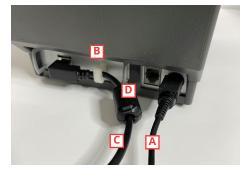
2. Connect the printer by plugging in the power cord A and USB cable C, using the white clip B to secure the cable. Attach the Ferrite clamp D about 1 inch away from the clip to close.
