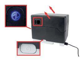
2. Press the printer power button on the left side of printer. A blue light will flash and stay lit. Push the lever on the right side of the printer to open lid.
