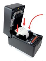
3. Press the blue lever and place in label roll facing upward in between the guides to adjust to label roll width.
