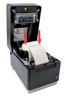
4. Gently push the label roll into the guides to insert shafts on each side of label roll to snap in place.
