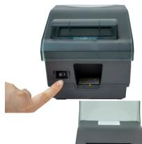
2. Press the printer power switch to the I position to turn on printer and light illuminate's green. Lift the splash cover and press the release button to open printer.
