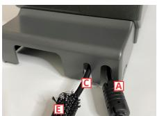
1. Connect printer power cord A to matching port on back of printer and to an outlet. Open white clip B and connect the USB cable C to the matching port feeding through the clip. Close clip and attach the Ferrite clamp D 1 inch from the clip. Snap the printer cable cover in place to protect connections. Attach the mesh cable protector E to the USB cable.
