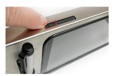
6. Press and hold tablet power button releasing when DateCodeGenie® displays.
