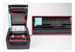
3. Gently pull the blue/green core bar from the right side and extend straight up. Slide the black line sensor to the far right of the opening.
