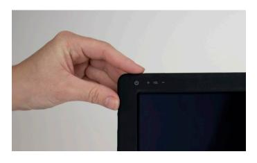
9. Press and hold tablet power button on top of silicone cover, releasing when DateCodeGenie® displays.
