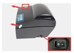
2. Press the printer power switch to the – position to turn on printer and light illuminates green. Pull forward on both blue/green levers to open the printer.
