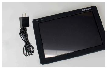
8. Attach tablet micro USB cable and tablet USB power adapter. Connect to port on tablet and an outlet and charge for 1 hour.
