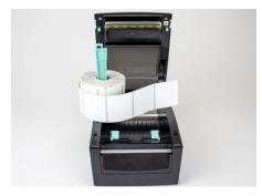
4. Slide the label roll on core bar with labels facing forward and unrolling from left. Snap the core bar closed.
