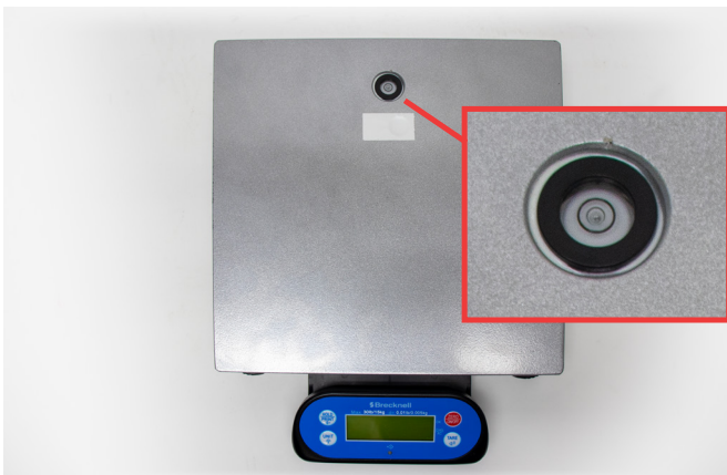
10. Place the scale in final location for use and view the level bubble. Adjust the feet until the bubble is centered.
