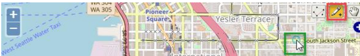
Figure 16: Using the Point Feature tool (red box) to specify the map center (circle inside green box)
