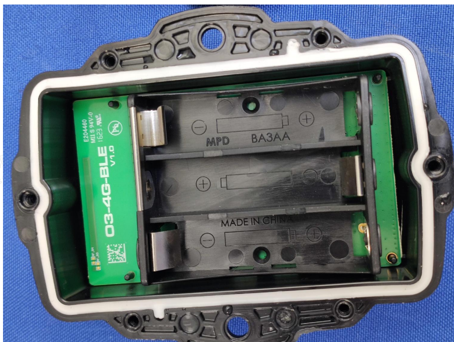
Photo 6: Test result of IP6X and IPX8 test
