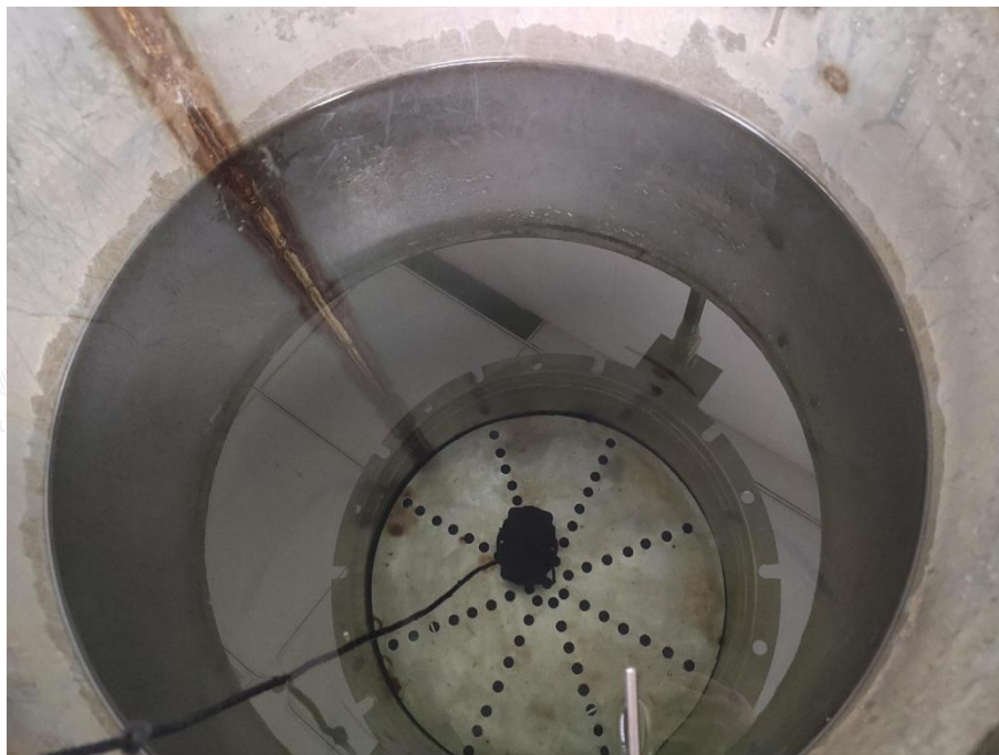
Photo 4: IPX8 test of model OYSTER3-4G
