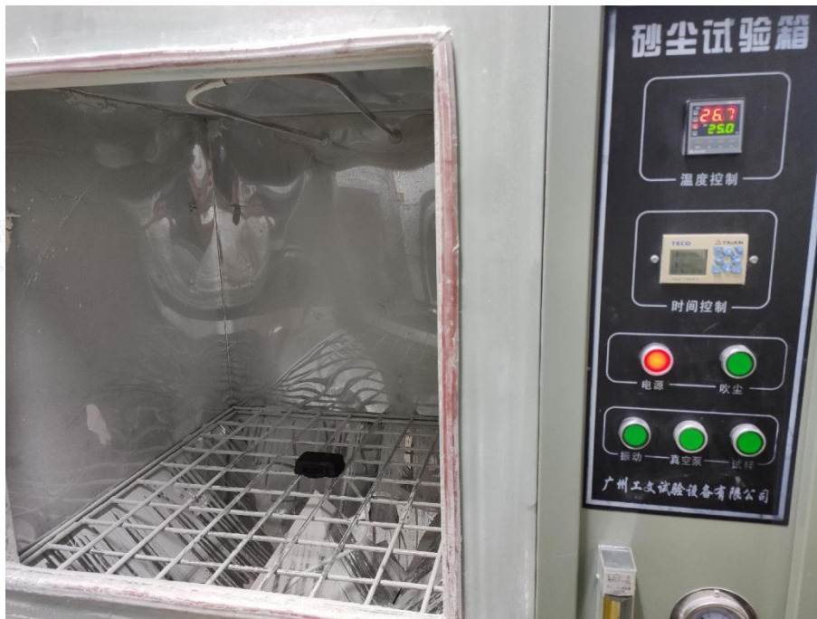
Photo 3: IP6X test of model OYSTER3-4G
