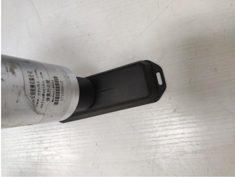
Photo 3: IK07 test of model Barra Clip
