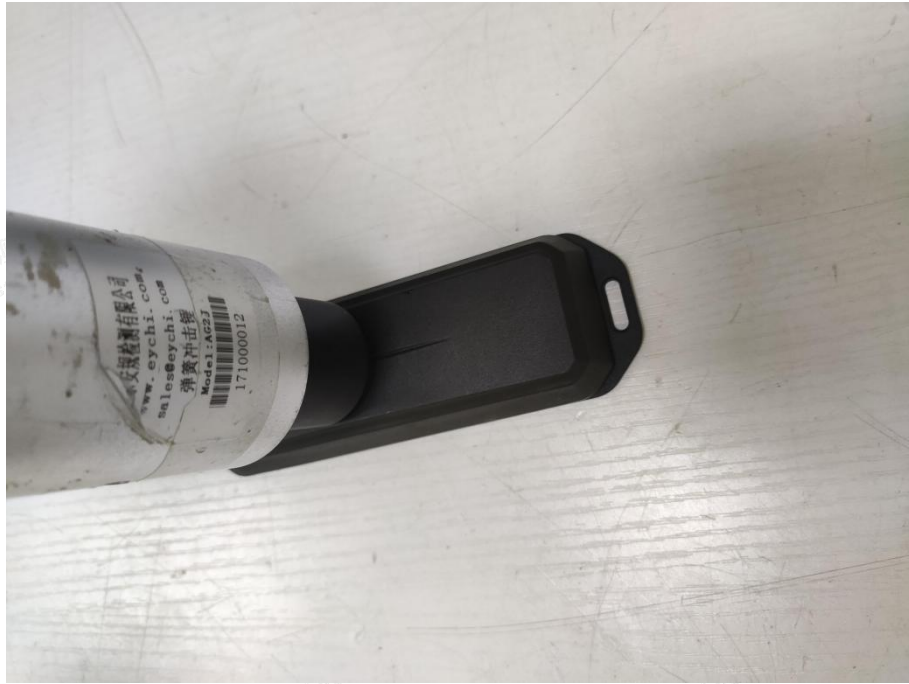
Photo 3: IK07 test of model Barra Clip
