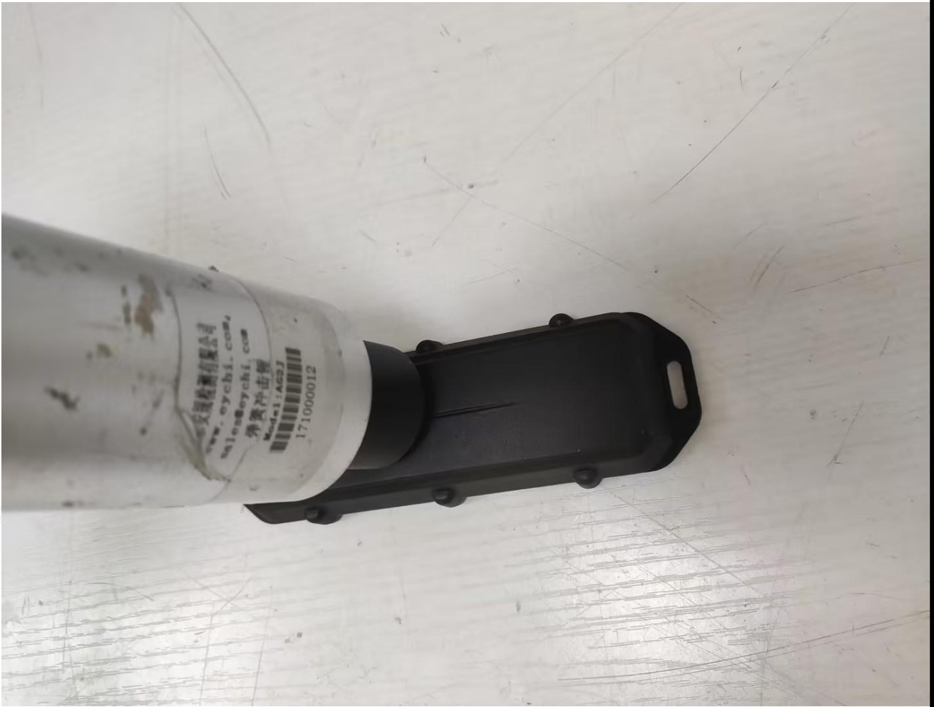
Photo 3: IK07 test of model Barra (Screw-type)
