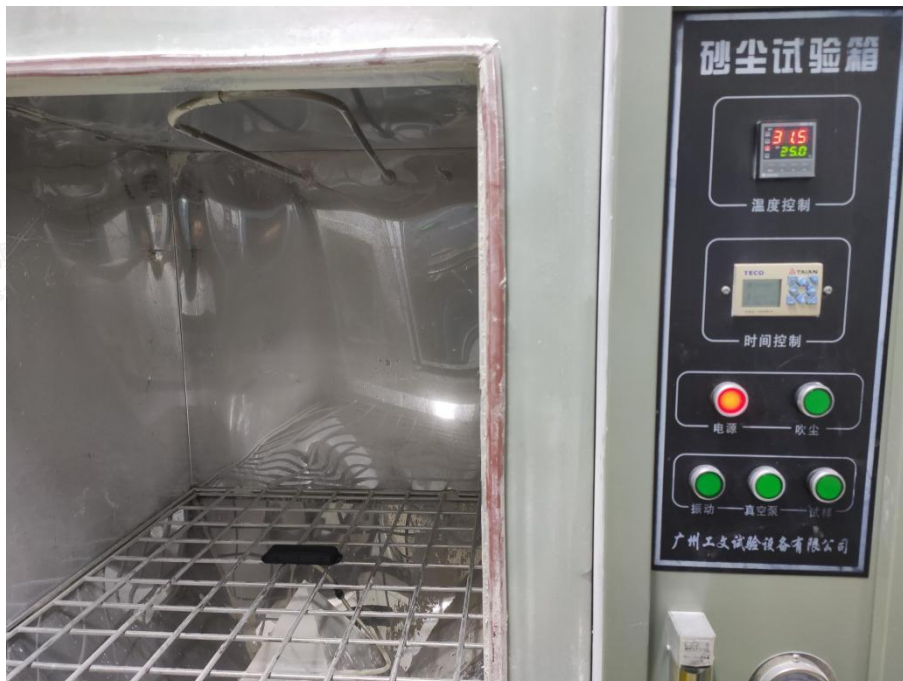
Photo 3: IP6X test of model Barra (Screw-type)
