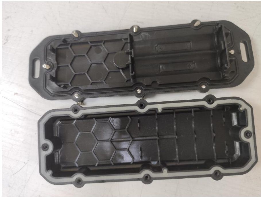
Photo 4: Test result of IP6X and IPX8 test
