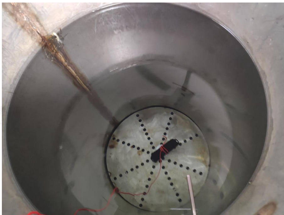
Photo 4: IPX8 test of model Barra (Screw-type)
