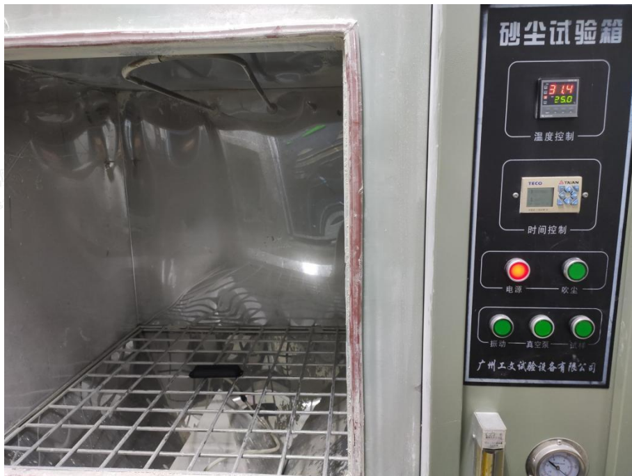
Photo 3: IP6X test of model Barra Clip
