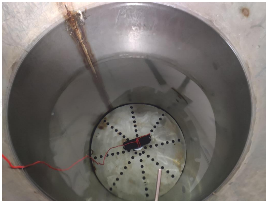
Photo 4: IPX8 test of model Barra Clip
