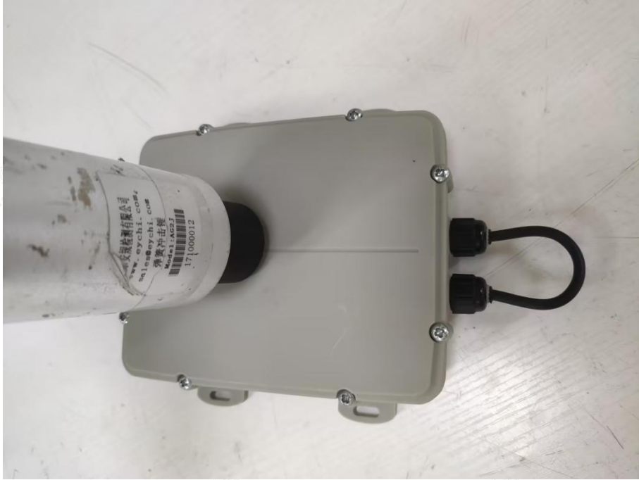
Photo 3: IK07 test of model HAWK 2D
