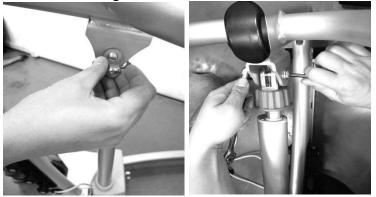
9. Install the control box onto the mounting bracket on the mast, and tighten the control box with two mounting screws (M4).
