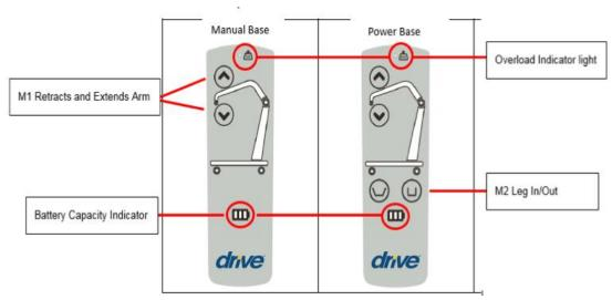
Definitions: M1 -Actuators for Lifting;
