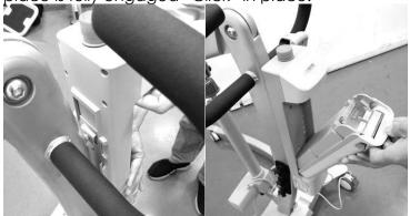
11. Plug the handset and actuator cables into the socket located on the bottom side of control box. Refer to the figures below for correct positions.
