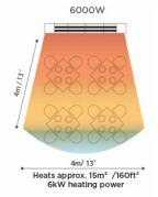
\*Heating areas are based on protected environment with mounting height of 96" (8'). For unprotected and extremely cold and windy environments heating areas can be less. Please contact Bromic Heating for further advice.
