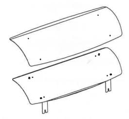
Turn Heat Deflector over and attach Outer Skin to Inner Skin using 4xM4 screws provided.
