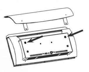
Mount Heat Deflector to back of heater by loosening the two screws and secure brackets underneath washers.
