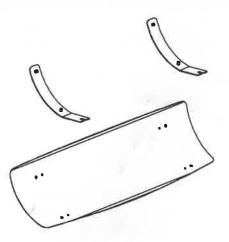
Attach Mounting Brackets to Inner Skin of Heat Deflector using 4xM4 screws provided.
