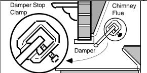
1. The chimney damper must be fixed in a manner to maintain a permanent free opening of at **least 39 square inches** based on a minimum chimney height of at least 8 feet. The area of the flue must not be less than 1/10 the area of the fireplace opening. **The flue must exhaust all products of combustion. MINIMUM PERMANENT CHIMNEY OPENING** is accomplished by either installing the provided damper clamp, permanently fixing the damper open, or by drilling holes in the damper blade.
