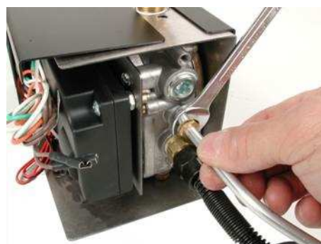
Figure 16 Tighten Pilot fitting with 7/16" end wrench or adjustable wrench. Push in on tubing while tightening.
