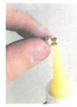
Replace manifold and fasten with the four mounting screws.
