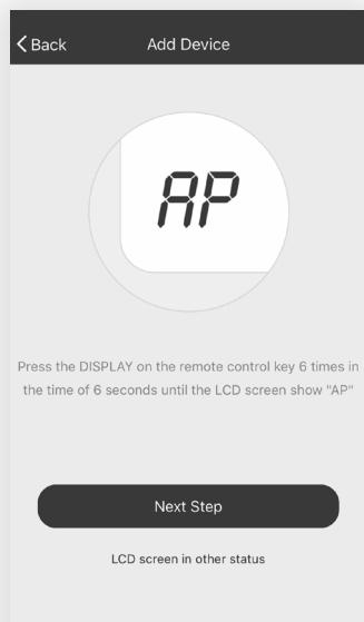
3. To switch the AC unit over to AP mode - Press “Display” on the remote control 6 times within 6 seconds so the AC unit switches from “CF mode” to “AP mode”. Allow the unit 10-15 seconds to switch modes and AP will flash on the AC unit display screen when complete.
