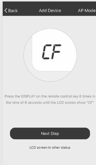
**Note:** If the AC unit is not in CF mode, press Display on the remote 6 times. After 8 to 10 seconds your will hear two beeps and the AC will display CF.
