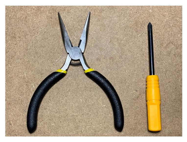
You will need Needle-nose Pliers and a Phillips head Screw Driver to complete this task.
