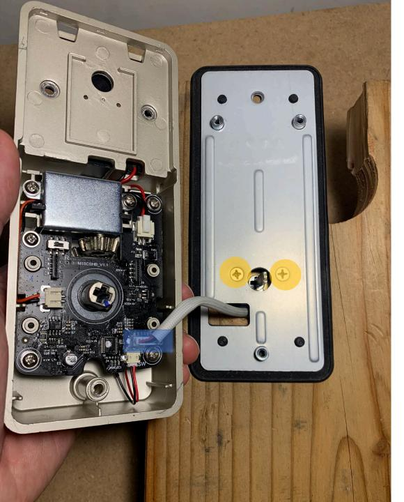
Loosen and remove the two Phillips head screws that secure the Lock Front Assembly (highlighted in orange).
