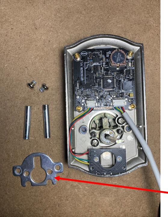
Remove the metal plate. The Key Cylinder is now free and ready to be replaced.
