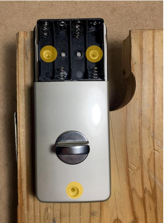
Re-attach the three Phillips head screws that hold in the Lock Back Assembly (highlighted in orange). Re-install AA batteries, and your lock is ready to use!
