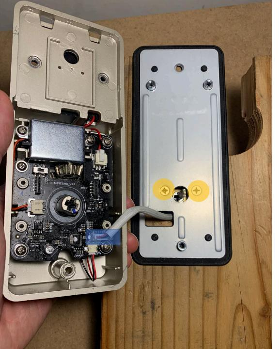
Re-attach the two Phillips head screws that secure the Lock Front Assembly (highlighted in orange).
