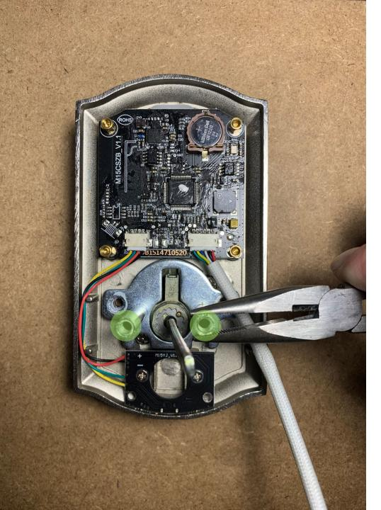
Loosen and remove the two threaded spacers (highlighted in green). Grip the spacers with a pair of pliers on the flat sides near the top, then rotate counterclockwise to loosen.
