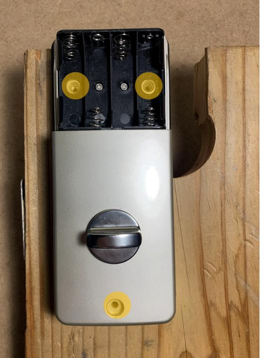
Remove the AA batteries. Loosen and remove the three Phillips head screws that hold in the Lock Back Assembly (highlighted in orange).
