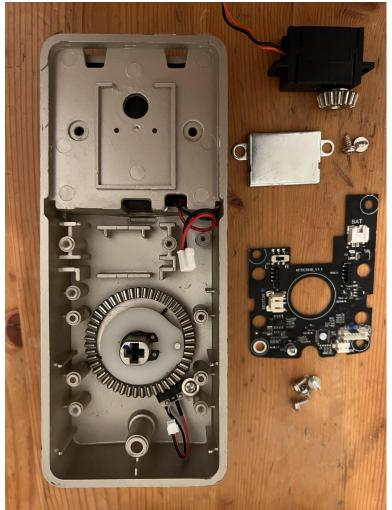
There are two screws that secure the motor in place
