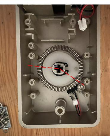
If the spring arms on the large gear are not in the correct starting position, the lock will not function properly. One example of an incorrect starting position is shown in red. The large gear must be in the orientation shown in green when installed.
