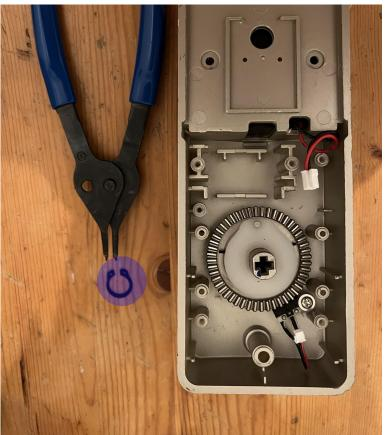
To reposition the actuation pin, start by removing the retaining ring with a pair of retaining ring pliers.
