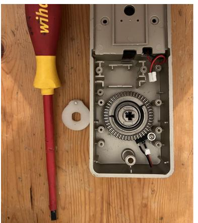
Once the ring is removed, the entire white plastic piece can be removed.
