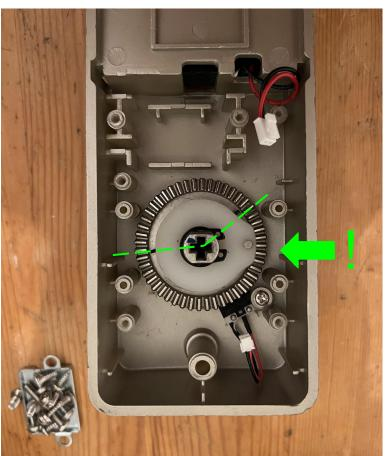
Place the white plastic piece with the actuation pin located within the large angle of the spring arms as shown. It is fully set when it clicks into place.
