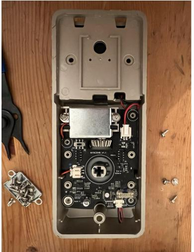
Remove the Back Plate from the MojoLock; this will expose the circuit board and motor.
