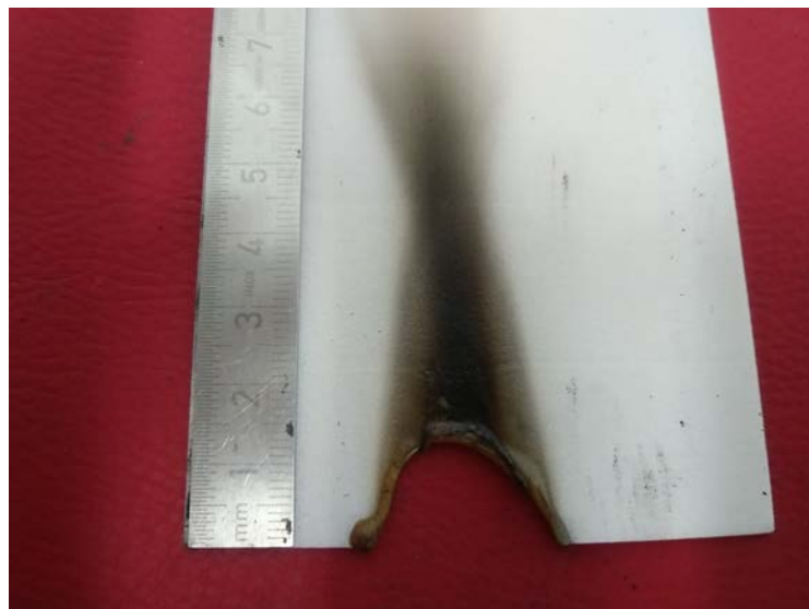
1/F19070 - Burnt area detail view
