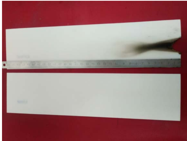
Comparison between burnt sample 1/F10970 and non burnt sample 2/F19070
