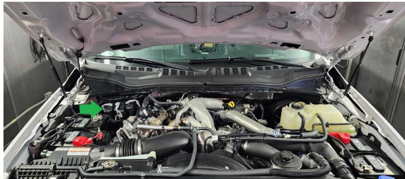
4. Be sure to release the locking tab (green arrow below) before moving gray connector arm. Disconnect all 3 of the ECU connectors.
