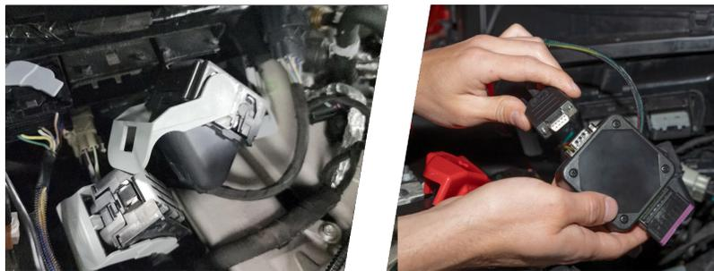
6. Connect the BDX to the Bully Dog box using the OBDII cable.
