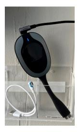
Connect the HDMI dongle to your computer, either by directly connecting to the computer or by using the HDMI adapter. A blue light will appear at the end of the dongle, and within 20-30 seconds the screen will start presenting your device. Tip: Do not press the dongle button, just wait.
