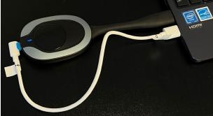
Connect USB-C to transmitter and connect the other end to the dongle or directly to the computer.
