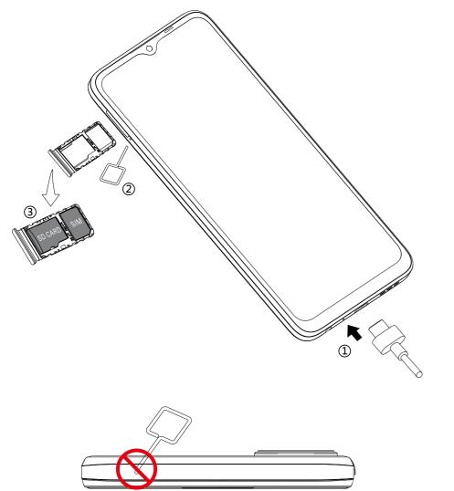
Caution: Do not insert the SIM pin into the small holes on top or bottom of the phone.
