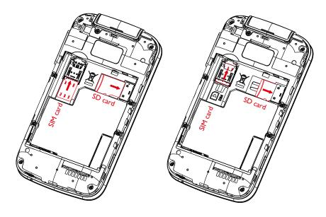
To remove the SIM card or microSD card, press down on the small plastic tab (1), then slide out the card (2). Do not use force or use any sharp objects.
