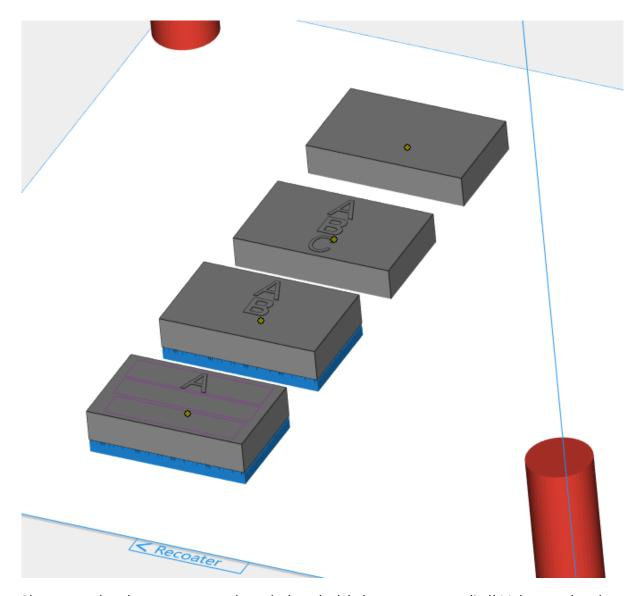
Please note that the supports are adopted when the label contents are applied! Make sure that the functionality of the supports is not impaired by the applied label content and the modified part surface.
