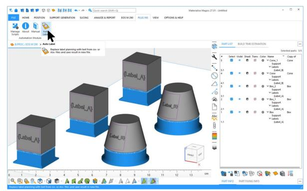
A dialog appears in which a profile can be selected, and parameters can be adjusted. Select the profile to be used and press the "EXECUTE" button to start automatic labeling.
