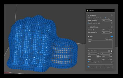
Introducing the organic sinter box that wraps tightly around your parts
