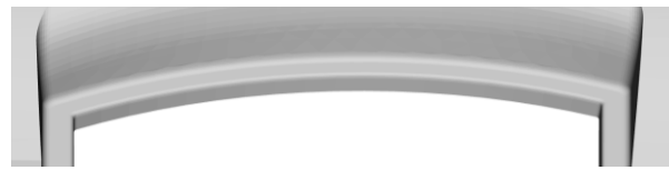
Output of Fillet operation on multiple contours
