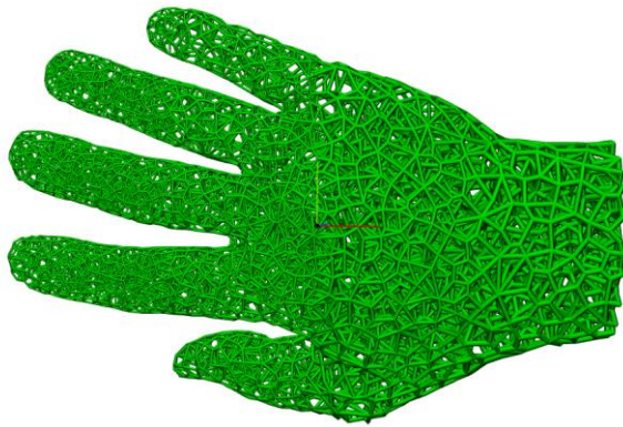
Voronoi based lattice structure with gradient density (the range of pore sizes [1.5-5mm])
