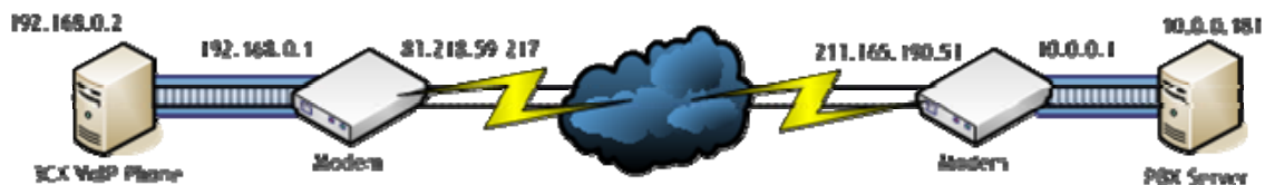
Figure 4 - How a tunnel works
