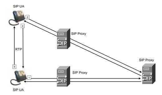
In a SIP VoIP network, when the SIP proxy receives a request from a UAS for a connection and it does not know the location of the UAC, it forwards the message to another SIP proxy in the network. Once the UAC is located and the response is routed back to the UAS, a direct peer-to-peer session is established between the two UAs. The actual voice traffic is transmitted between UAs over dynamically assigned ports using the Real-time Protocol (RTP).
