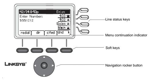
The function of the four soft keys depends on the option appearing on the LCD display. When more than four functions are available, a small left or right-facing triangle (menu continuation indicator) appears at the bottom of the LCD display. This indicates that more soft key functions can be accessed by pressing the **Navigation** button left or right.
