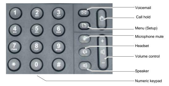
To use the shortcut to an option, press the **Menu** (Setup) button and type the number assigned to the option. The option does not have to appear on the LCD to use the shortcut. To select an option with a two-digit shortcut, press the second number within two seconds of the first number.
