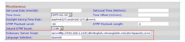
During startup, the phone checks the selected/preferred language and downloads the dictionary from the TFTP/HFTP provisioning server indicated in the device configuration. The dictionaries are available at the following website:
