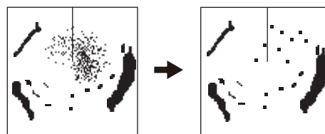
Rain clutter (starboard direction) A/C Rain adjusted; rain clutter suppressed.
