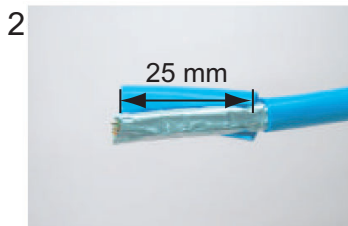
2 Remove the inner vinyl sheath by approx 25 mm. Be careful not to damage inner shield and cores.
