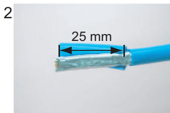
Remove the sheath by approx 25 mm. Be careful not to damage inner shield and cores.
