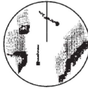
(b) Relative target trails Targets moving relative to own ship
