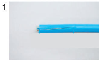
1 Expose inner vinyl sheath.
