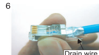
6 Insert the cable into the modular plug so that the folded part of the shield enters into the plug housing. The drain wire should be located on the tab side of the jack.
