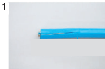
Expose inner vinyl sheath.
