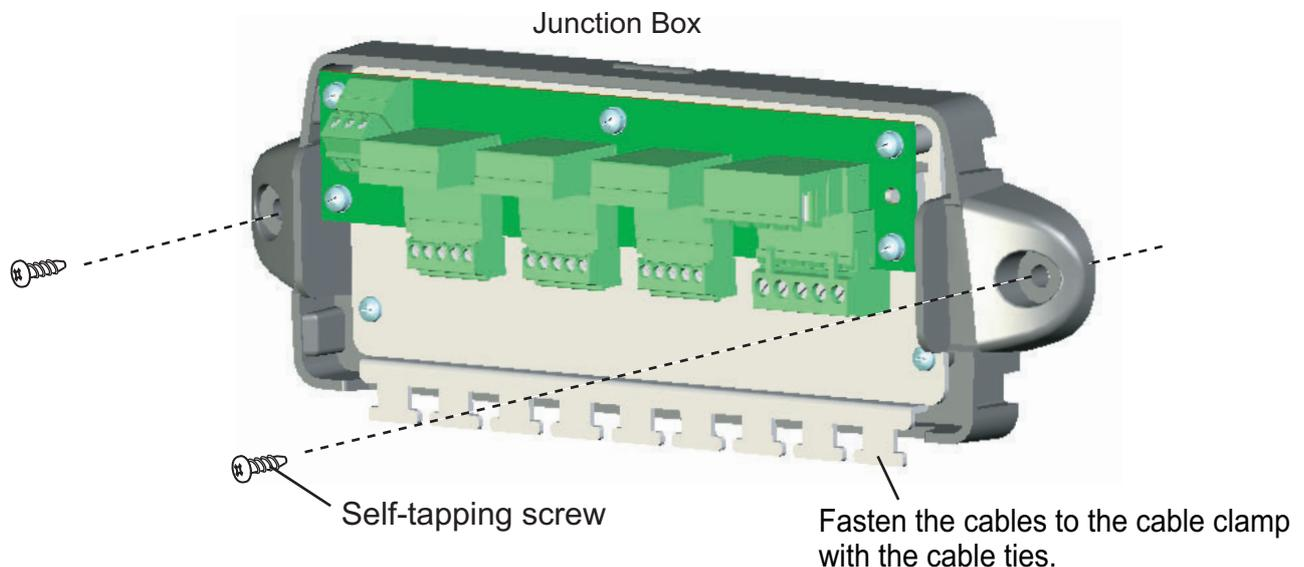
3. Connect the cables to applicable connector, referring to the interconnection diagram provided in the operator's manual or installation manual of a device connected to the Junction Box.
