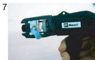
7 Using the special crimping tool MPT5-8 (PANDUIT CORP.), crimp the modular plug. Finally, check the plug visually.
