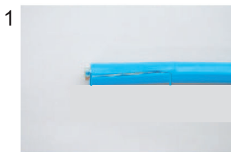
1 Expose inner vinyl sheath.
