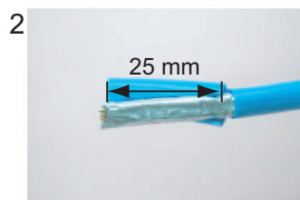
2 Remove the outer sheath by approx 25 mm. Be careful not to damage inner shield and cores.
