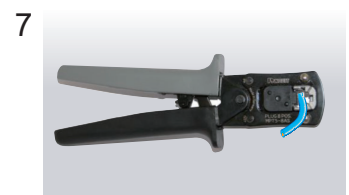
7 Using special crimping tool MPT5-8AS (PANDUIT CORP.), crimp the modular plug. Finally check the plug visually.
