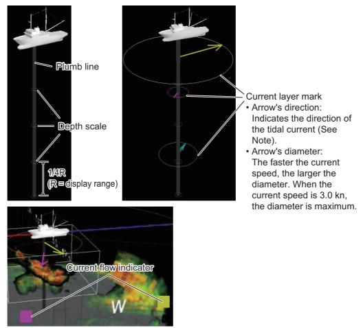
**Note:** Arrow's direction shows "from what direction the current is flowing" or "the direction the current is heading". [5 Current Flow Dir] on the [Current VEC & Wind]menu selects from what direction to display current data. See section 9.2.6.
