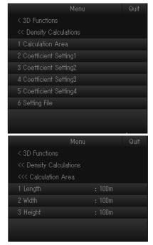
5. Adjust the values for [1 Length], [2 Width] and [3 Height] to adjust the calculation area size.
