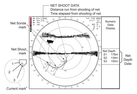
\*: The current mark can be shown/hidden from [4 On Net Shoot Mark] (located at main menu  $\rightarrow$  [0 Mark & Operation Support Tool]  $\rightarrow$  [6 Net Course Mark]). See section 9.2.6.
