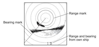
**Note 1:** You can clear the range and bearing marks and the indications at the bottom of the screen. Place the cursor on, or near, the own ship symbol, then press the **R/B AUDIO** key.
