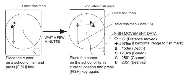
**Note 1:** The time and distance between each press of the **FISH** key should be as long as possible to increase accuracy of measurement. For best results, repeat the procedure two or three times.
