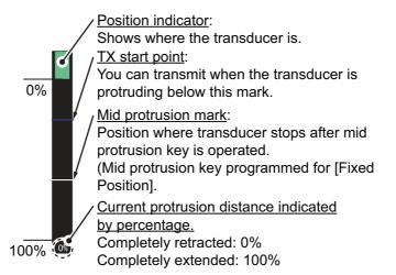
The color of the indicator changes according to transducer position and operation state.
