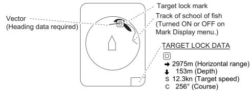
4. To disable the target lock, press the TARGET LOCK key.
