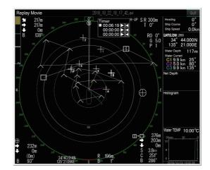
Controls for stopping playback, fast forwarding and rewind are provided on the [Motion Image] window.
