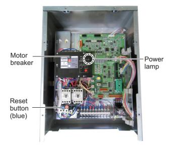
6. Push the RESET button (blue) on the raise/lower control box.
