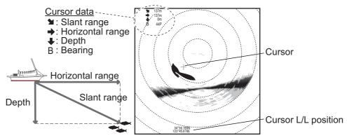
2. To measure the range and bearing to a different target, or mark the current target with its range and bearing, push the **R/B AUDIO** key. A range mark and bearing mark appear, intersecting the location selected at step 1. Further, the range and bearing to the target appear at the bottom of the screen.
