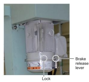
3. Remove the brake release level with a set of pliers.
