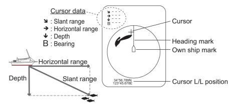
2. To measure the range and bearing to a different target, or mark the current target with its range and bearing, push the **R/B AUDIO** key. A range mark and bearing mark appear, intersecting the location selected at step 1. Further, the range and bearing to the target appear at the bottom of the screen.
