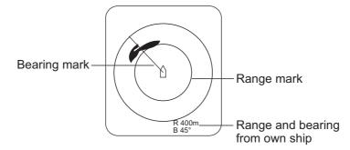
**Note 1:** You can clear the range and bearing marks and the indications at the bottom of the screen. Place the cursor on, or near, the own ship symbol, then press the **R/B AUDIO** key.
