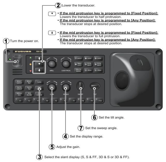
**Note:** In the default setting, Slant (S) and Vertical Slant (VCS) modes are active. To use other display modes, register the display mode to use from the menu. For how to register display modes, see section 1.6.2.
