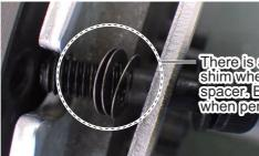
There is a chance to drop the shim when you remove the spacer. Be sure to catch the shim when performing this operation.
