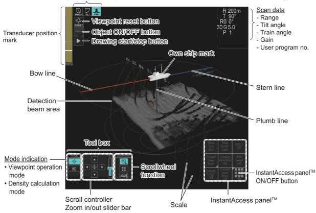
**Note 1:** The display expand/retract button, which expands, retracts the display in the 3D & S mode, is not shown in the default configuration. To show the button, [1 2nd Monitor Setting] on the [Monitor Setting] menu (see page 9-12) must be set to [Sub Display] or [OFF]. The button appears below the drawing start/stop button.
