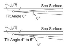
This causes one half of the emitted sound to be reflected toward the transducer and displayed on the screen as sea surface reflections. When the sea is calm, since the sound is reflected just like a light hitting a mirror at a low incident angle, it propagates away and the sea surface reflections become negligible.
