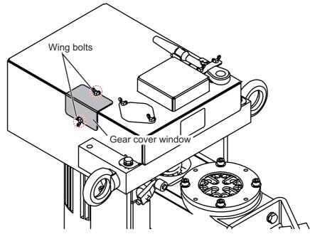
2. While raising and lowering the transducer manually with the ratchet wrench (see section 10.11.2), apply Molytone No.2 Grease.
