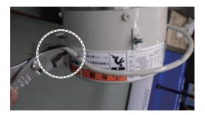
4. Remove the brake release lever pin with a pair of pliers.
