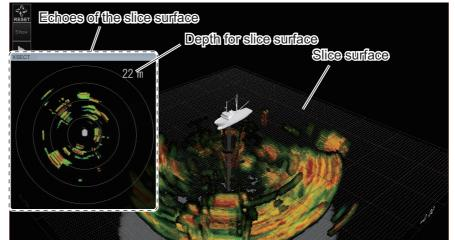
• [1 Cross-Section Movement] = [Scale-Based]: Shows the slices that are vertical to the sea surface.
