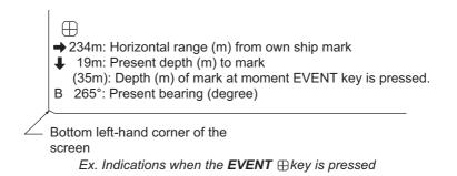
With speed and heading data the mark follows own ship's movements. When the tilt angle is changed, the present depth to event mark changes. Note however that the mark's position does not change when automatic tilt is active; the tilt center angle is used to position the mark.
