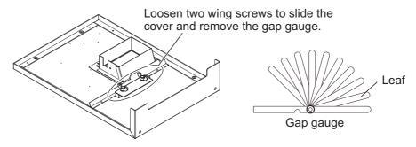
Insert the leaf of the gap gauge horizontally to the place of measurement. Take the measurement. Measure the gap at three places.
