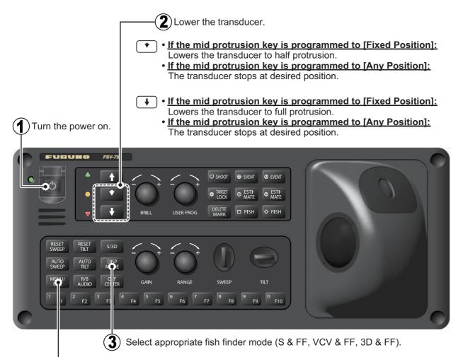
(A) Adjust reange, gain and picture advanse speed on the menu.
