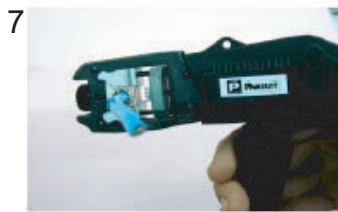
Using special crimping tool MPT5-8AS (PANDUIT CORP.), crimp the modular plug. Finally check the plug visually.
